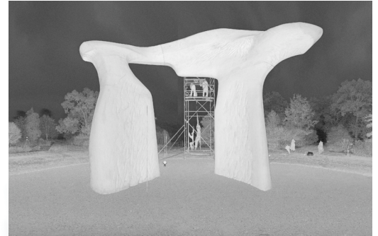
The complete 3D dataset captured from the fibreglass Arch at RHS Wisley
