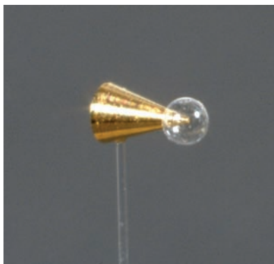
Typical products include a gold cone and plastic shell (left) for fusion research and a thin foil on an aluminium assembly (right) for generation of particle beams for cancer therapy.
