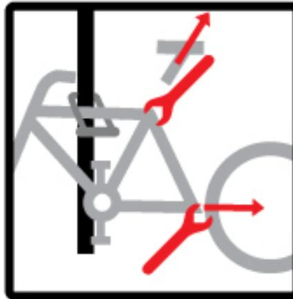
Always lock both wheels and the frame of your bike to the stand and remove any quick release accessories such as saddle and wheels. If you only wish to carry one lock then secure skewers are a good idea. These are available from most good cycle shops and do not allow unauthorised removal of wheels, meaning you only need to secure your frame to the stand.
