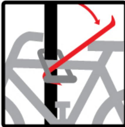
Always fit your lock so that as much of the aperture within the lock is filled by the stand and bike (and maybe helmet). This will make it harder to insert tools between the lock and the stand. **Never lock your bike by the 'top tube' (AKA 'crossbar') alone** as this will allow for the bike frame to be rotated against the lock.
