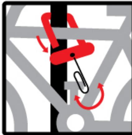
Most good locks are designed to resist this technique. Check that yours is one of them. Also, make it harder for the would-be thief by securing your lock in such a way that the mechanism is hard to get at. Tightly secured to the bike and stand and facing into your bike. Whilst this makes things a little more difficult for you it will make it a lot more difficult for a lock picker.
