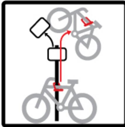
Always lock your bicycle to a 'closed structure' that is well secured to the ground. If you must lock to an 'unclosed structure' then make sure it is more than 5 metres high and well secured to the ground (thieves will stand on shoulders to pass your bike clear if the structure is low enough).
