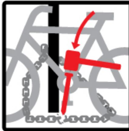
Always ensure your lock is fitted so that it cannot rest upon the ground or other immovable surface. This will allow the lock or chain to move if it is struck, diffusing the force of the strike and keeping your lock or chain in one piece.
