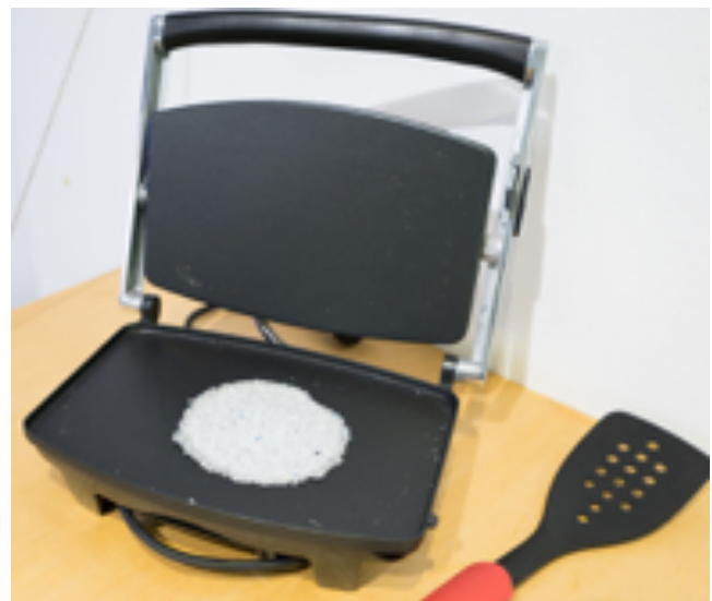
Figure 6. Household sandwich press and heat formed tiles from loose pulverised fluff
