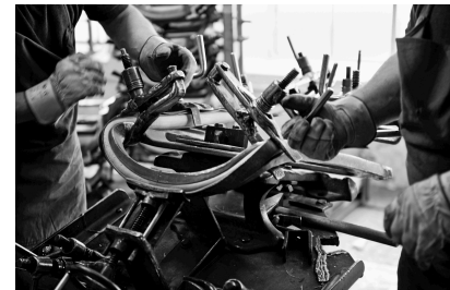
Fig. 6: A contemporary photo of the Thonet jig-bending process developed in the 19 th century, still in use (photo credit: Thonet/Claus Setzer). The extreme curves achievable by this method were not previously possible without ply-construction
