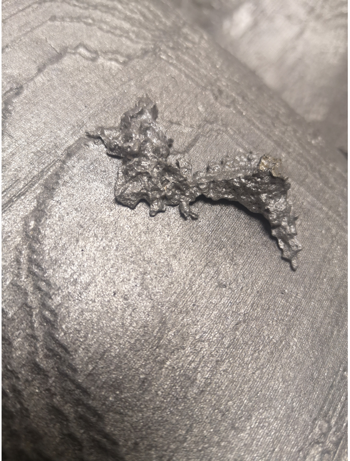
Image 35: Digital photograph of flashing on the surface of the aluminium sculpture.
