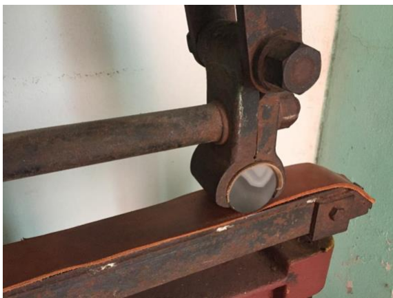
Fig 10: Polishing machine with a mechanical arm and a cylindrical agate stone
