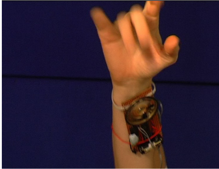
Figure 16. Bourdon - Gestural action with wrist speaker activating/de-activating tilt switch to make or break the sounding circuit, Interaktionslabor, Germany, 2011. Video still © Interaktionslabor/DAP-Lab.
