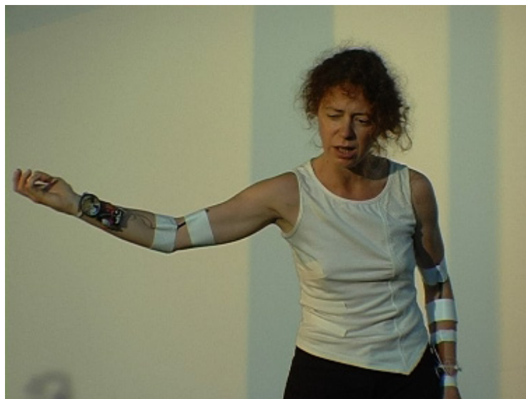
Figure 15. Bourdon - Sosana Marcelino explores the wrist speaker prototypes, each with inbuilt circuitry, accelerometer and tilt switch for motion sensing, attached to her left and right arms, Interaktionslabor, Germany, 2011. Video still © Interaktionslabor/DAP-Lab.
