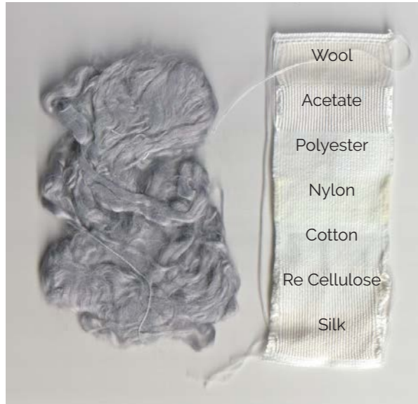
Appendix Figure 17: Sample 1 BCS wash-fastness test strip.
