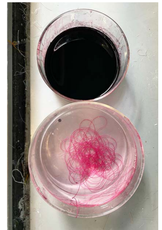
Figure 120: In-situ dye test 3 - filament results.
