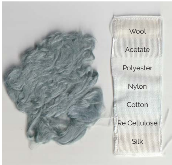
Appendix Figure 12: Sample 10 BCP wash-fastness test strip.
