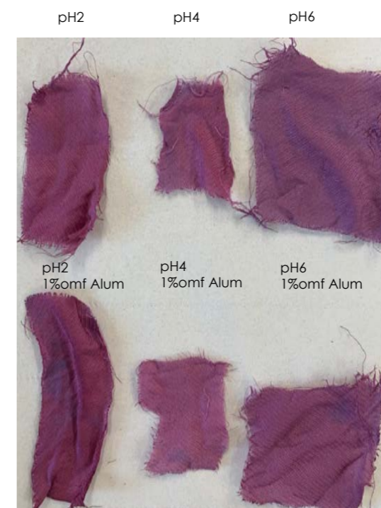
Appendix Figure 16: Casein fabric dyed with BCS, comparison of colour before washing.
