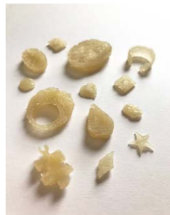
Figure 38: Test 1 - Extraction of casein from milk.
