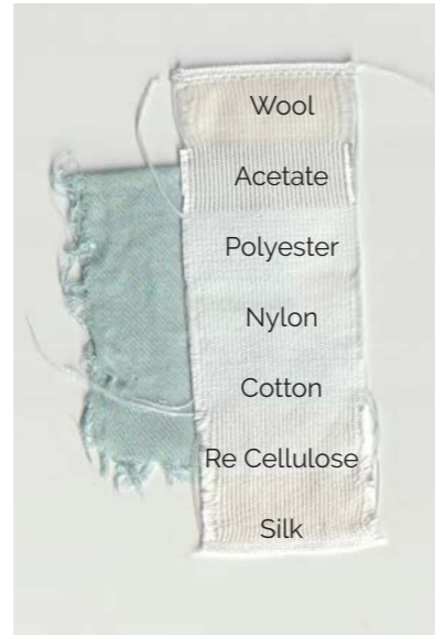
Appendix Figure 13: Sample 11 BCP wash-fastness test strip.
