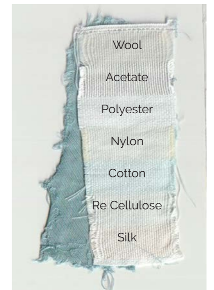
Appendix Figure 24: Sample 8 BCS wash-fastness test strip.
