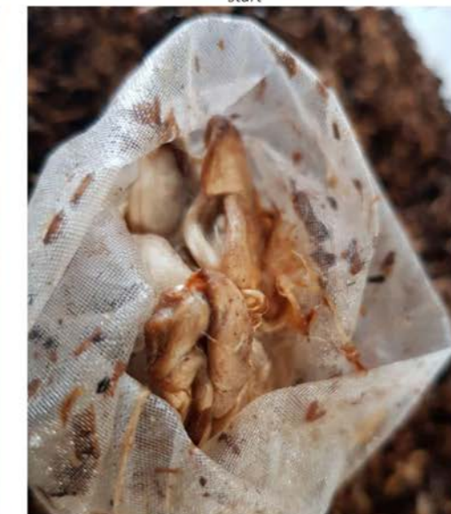
Figure 4: Samples at Day 49 showing detail of discolouration and compression
