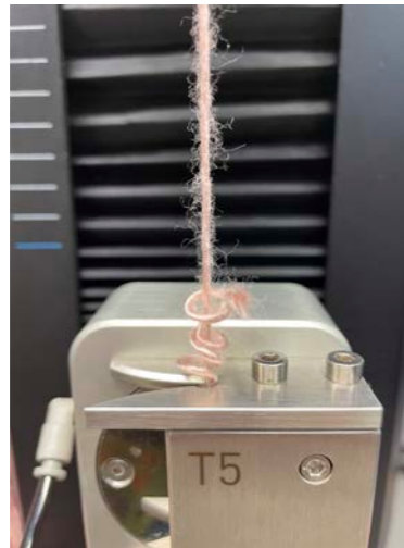
Figure 132: Tensile testing of commercial casien yarn - avocado dyed
