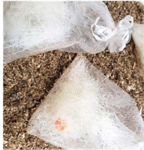
Figure 2: Sample and synthetic compost at start. Samples were placed in bags to track degradation.
