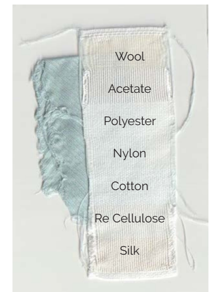
Appendix Figure 10: Sample 8 BCP wash-fastness test strip.
