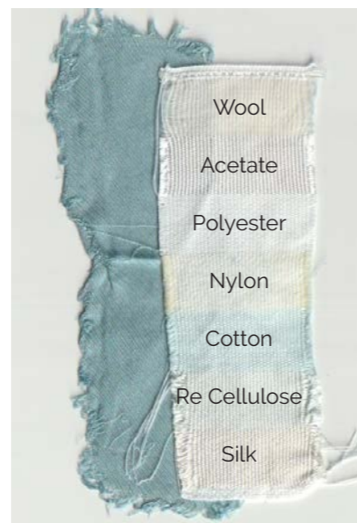
Appendix Figure 20: Sample 4 BCS wash-fastness test strip.
