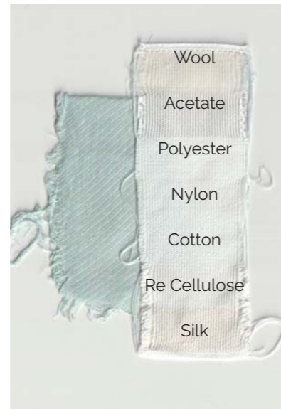
Appendix Figure 14: Sample 12 BCP wash-fastness test strip.
