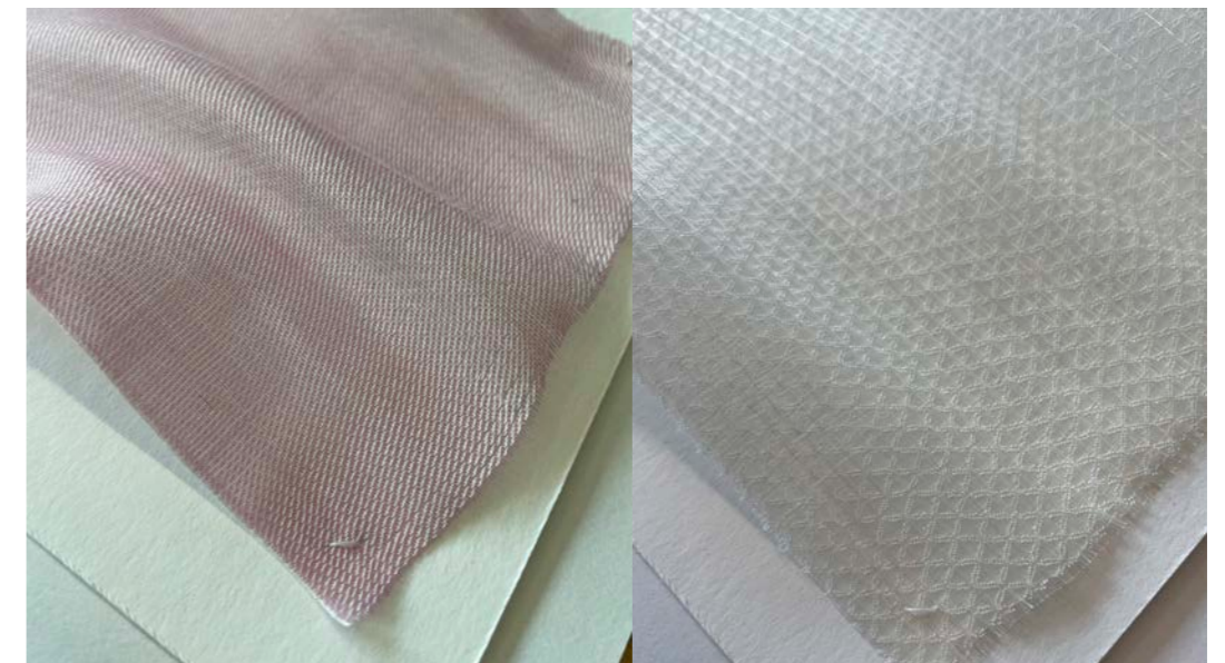
Figure 128: Woven monofilament Sample 1.
