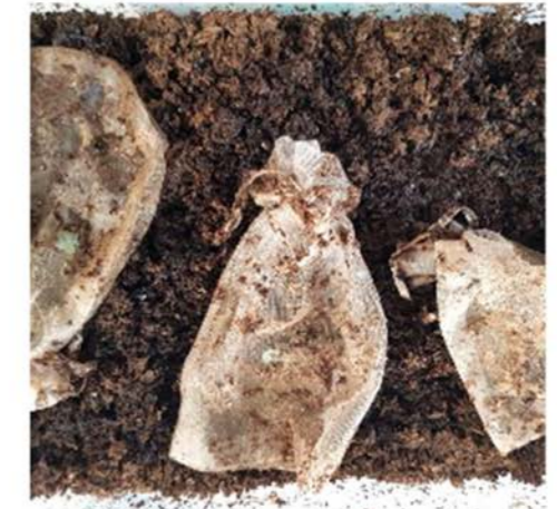
Figure 4: Sample at day 14 complete disintegration leaving empty bags.
