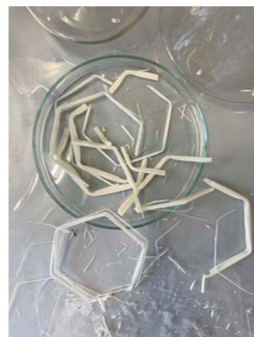
Figure 101: Hand winding of casein fibres onto various utensils for drying.
