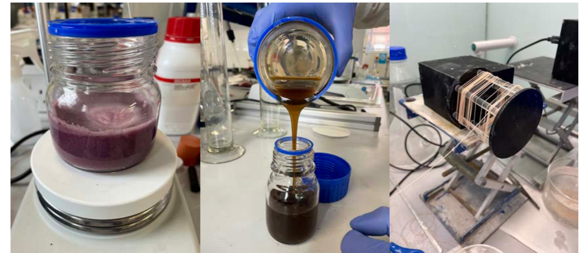
Figures 113 - 115: In-situ dye test 2 - preparation of dope and spinning of monofilament.
