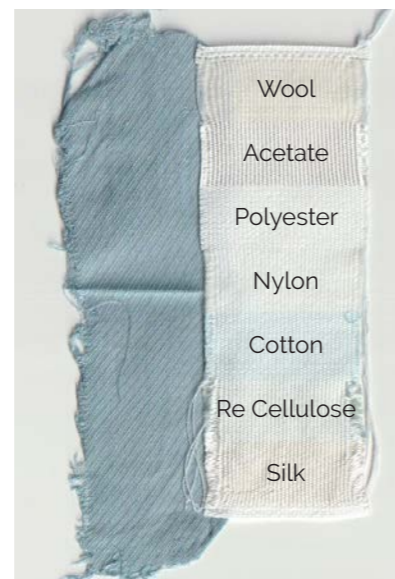
Appendix Figure 6: Sample 4 BCP wash-fastness test strip.
