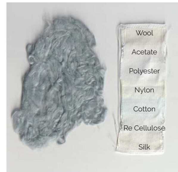
Appendix Figure 22: Sample 6 BCS wash-fastness test strip.
