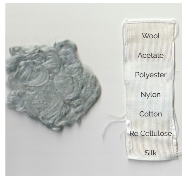
Appendix Figure 8: Sample 6 BCP wash-fastness test strip.
