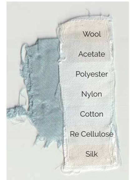
Appendix Figure 9: Sample 7 BCP wash-fastness test strip.
