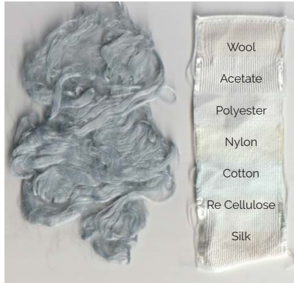
Appendix Figure 25: Sample 9 BCS wash-fastness test strip.
