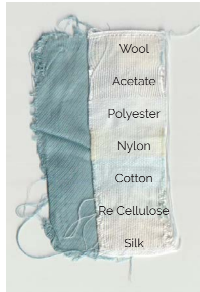
Appendix Figure 19: Sample 3 BCS wash-fastness test strip.
