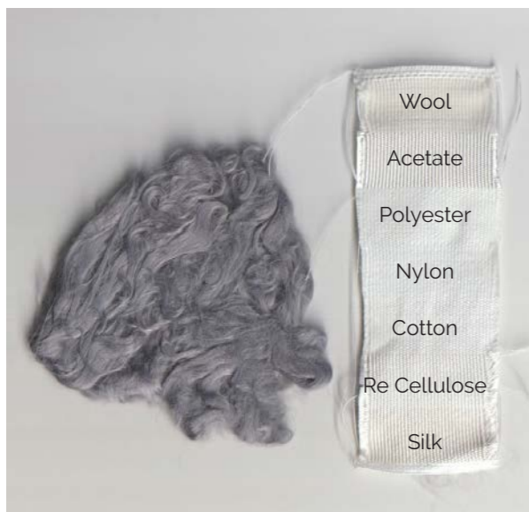
Appendix Figure 4: Sample 2 BCP wash-fastness test strip.
