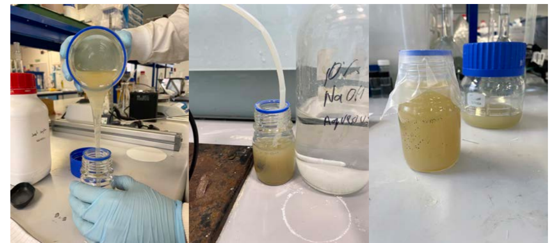
Figures 98-100: Preparation of casein dope for extrusion. The dope is thick yet pourable.
