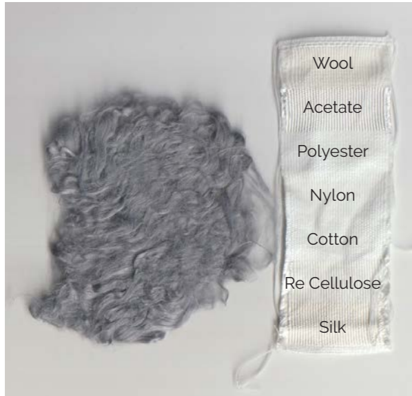
Appendix Figure 3: Sample 1 BCP wash-fastness test strip.
