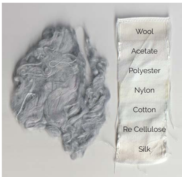
Appendix Figure 18: Sample 2 BCS wash-fastness test strip.
