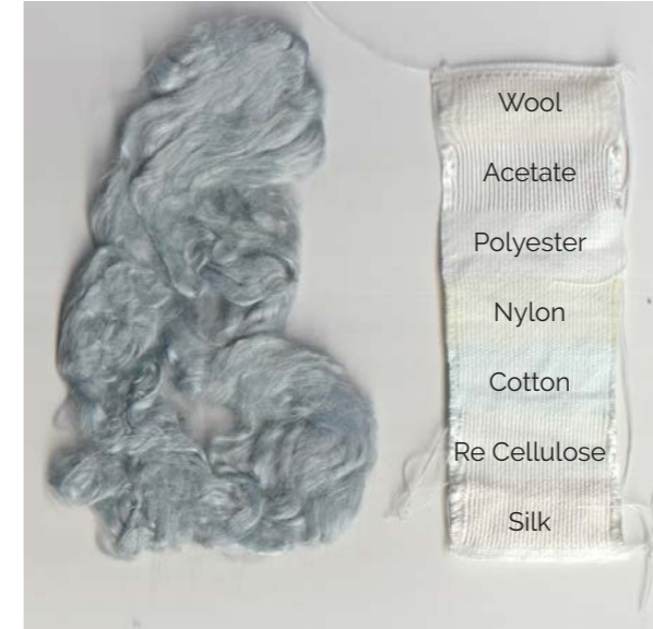
Appendix Figure 21: Sample 5 BCS wash-fastness test strip.
