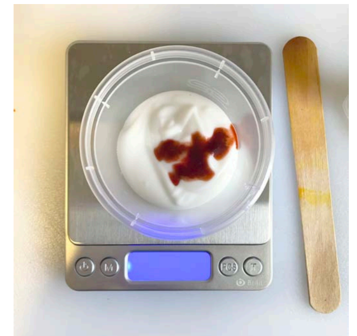
Figure 69: Preparation of SP3.2 (avocado ink) – mixing of reduced dye into Permaset).
