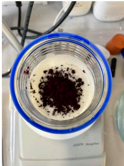
Figure 111: In-situ dye test 1 - Adding BCP to casein dope.
