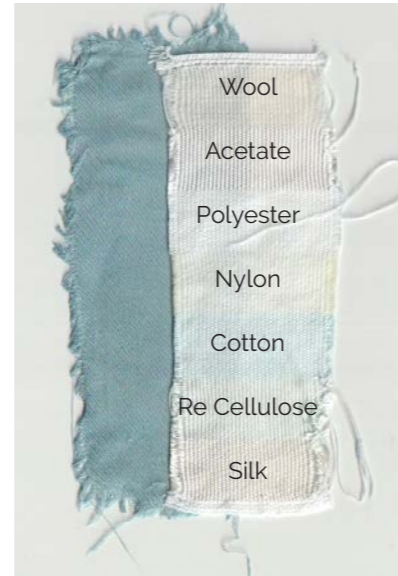
Appendix Figure 27: Sample 11 BCS wash-fastness test strip.
