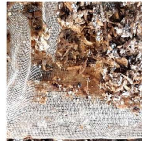
Figure 3: Samples at day 7 showing material dissolving and seeping through mesh.
