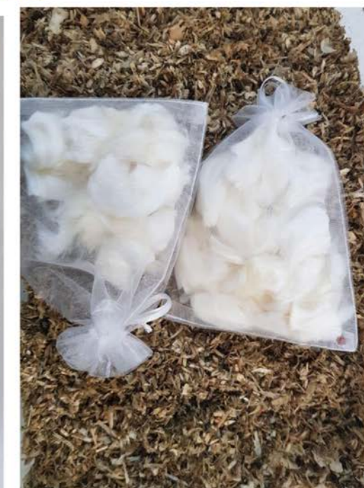
Figure 2: Samples in mesh bags on synthetic compost at the start
