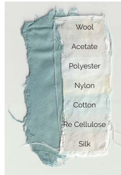
Appendix Figure 28: Sample 12 BCS wash-fastness test strip.
