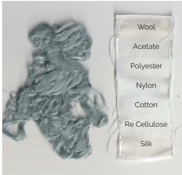
Appendix Figure 11: Sample 9 BCP wash-fastness test strip.
