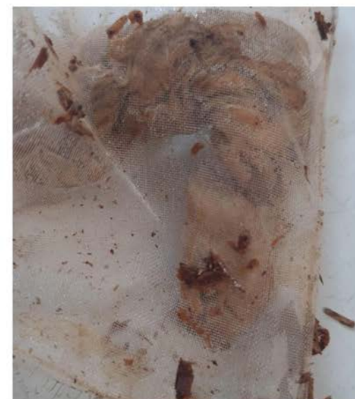
Figure 3: Samples at Day 28 showing compression and discolouration
