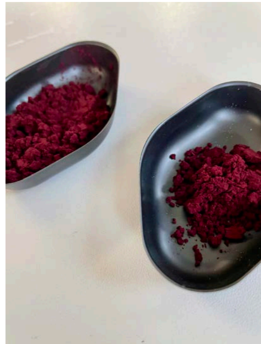
Figure 110: In-situ dye test 1 - Measuring of BCP.
