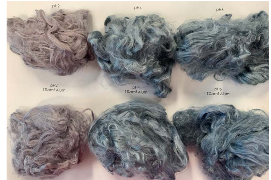
Appendix Figure 1: Casein yarns dyed with BCP, comparison of colour before washing.
