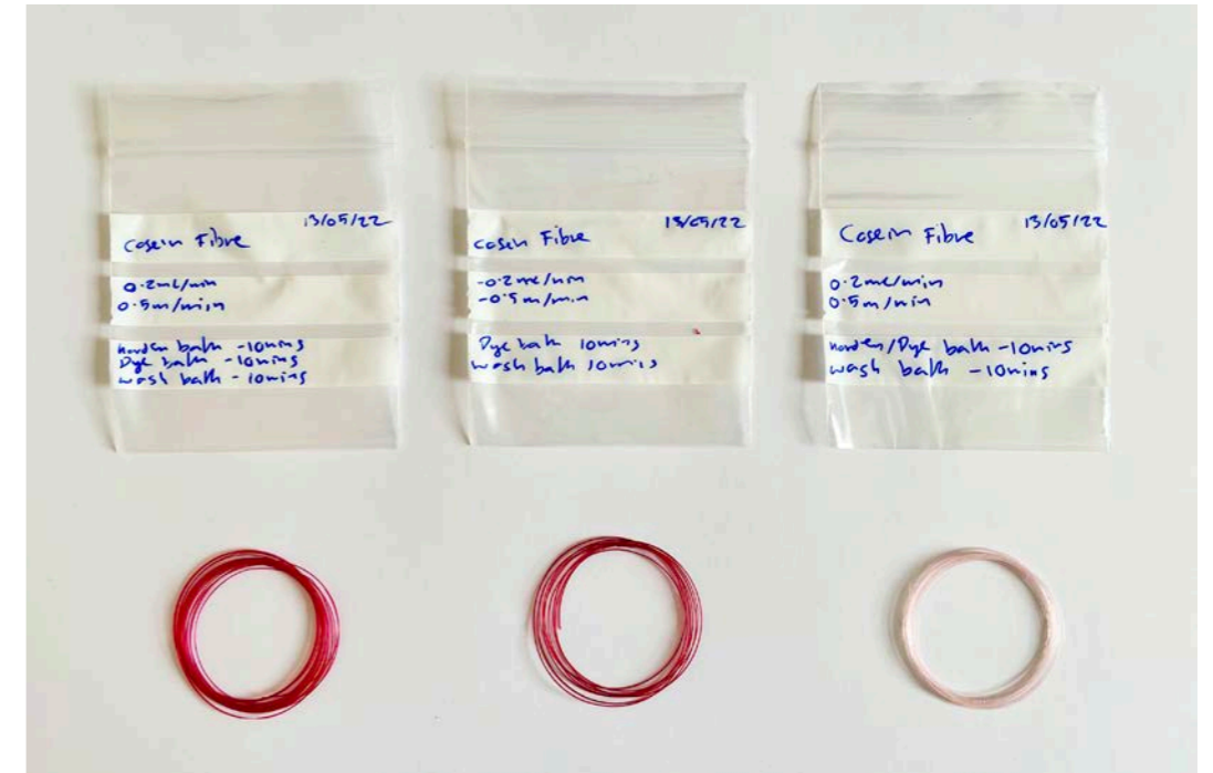
Figure 124: Comparison of colour between in-situ dye tests 3-4.
