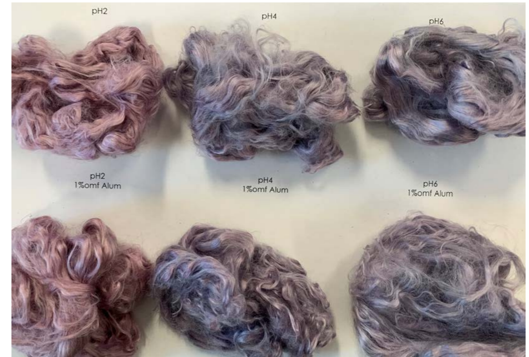
Appendix Figure 15: Casein yarns dyed with BCS, comparison of colour before washing.
