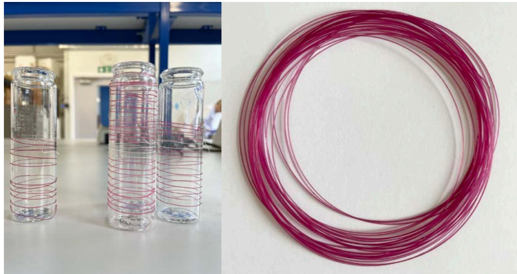
Figure 122: Hand wound filaments onto glass vials. Figure 123: In-situ dye test 4 - filament results.
