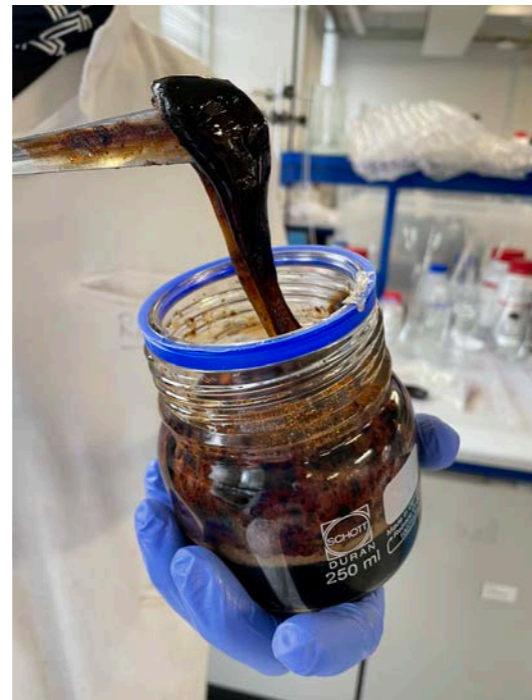
Figure 112: In-situ dye test 1 - Testing viscosity.
