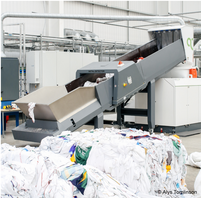
Polyester feedstock, including offcuts from products such as football shirts, ready for shredding and processing into recycled R-PET pellets.
