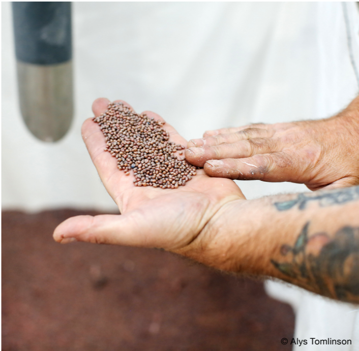
Pelletised R-PET made from post-consumer polyester waste.
