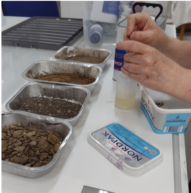
Fig 3. Preparing the clear glass resin with the thinner and activator.
