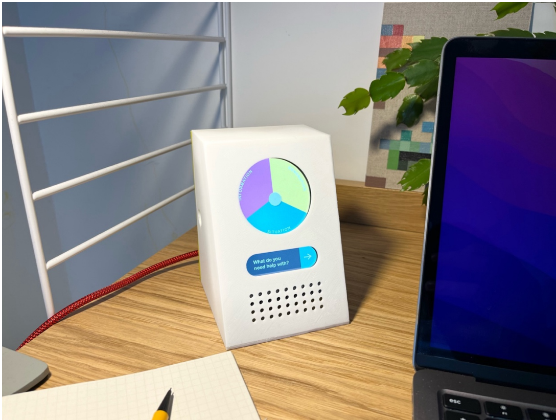
Figure 7.10: The Digital Probe Device on a desktop, powered on. A prototype version of the graphical interface is shown.
