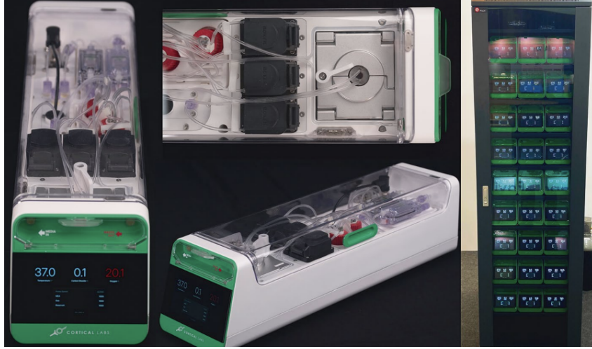
Figure 2: The CL1 biocomputer platform, showing the integrated microelectrode array (MEA) and perfusion system for maintaining neuronal cultures. Adapted from [9].
