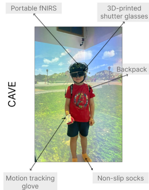
Fig. 9. Experimental setup in the CAVE. Participants wore a portable fNIRS system, consisting of two continuous wave fNIRS devices (Brite MKII, Artinis Medical Systems BV, Netherlands) mounted on a neoprene cap, a backpack for tucking away the fNIRS system's wires, a motion tracking glove for interacting with the virtual objects, custom-made 3D-printed shutter glasses allowing 3D vision, and non-slip socks to ensure safe and unrestricted in the CAVE.
