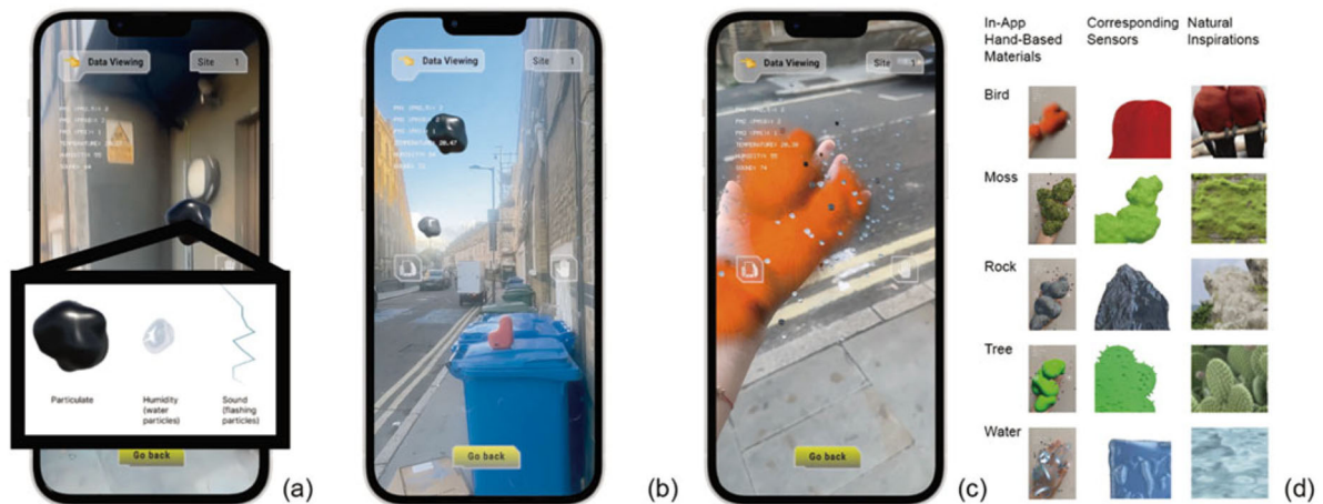
Figure 11. Screenshots of observation mode: (a) visualisation principles of different data types; (b) a screenshot showing collected data being physicalised in the AR interface; (c) users interacting with the physicalised data through gesture recognition; (d) overview of the in-app hand-based materials, their corresponding sensing devices, and the natural elements that inspired their form and material qualities.
