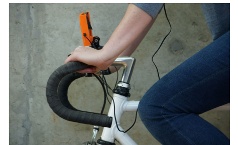
Jill Bennett, Volker Kuchelmeister and Laura Fisher Veloscape: a Curating Cities project, Data collection using galvanic skin response, go-pro camera and GPS, 2014. Photograph: Laura Fisher
