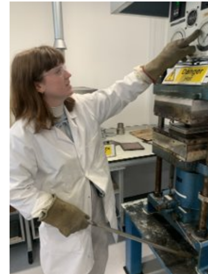
3. Hot press (10mins 2MPa) followed by water soak and air drying
