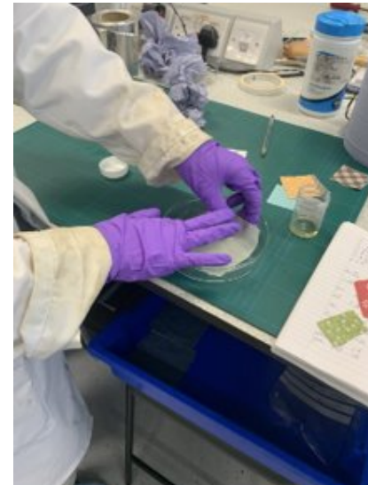
2. Soaking of cellulose materials in Ionic Liquid/DMSO solution (80:20)
