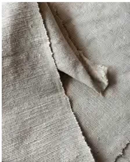
Circular Handspun fabric using Kala warp and recycled yarn weft Credit: Khamir
