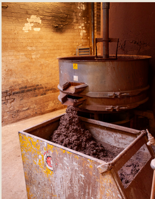
Fig. 2. Pan mixer, Valentine Clays, Stoke-on-Trent, 2015
