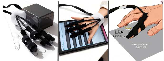
Fig. 1. RelicTouch: a fingertip haptic wearable system
