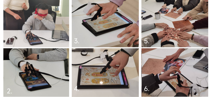
Fig. 7. Three experimental tasks. (1–2) Blind exploration: a participant located salient regions in a tablet-displayed image using vibrotactile cues. (3–4) Exploration of an engraved image using RelicTouch . (5–6) Comparison between printed texture samples and RelicTouch -based image exploration.
