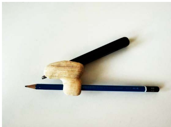
Figure 25 Photograph of the otoscope mounted to the pencil in a custom made wooden cradle.
