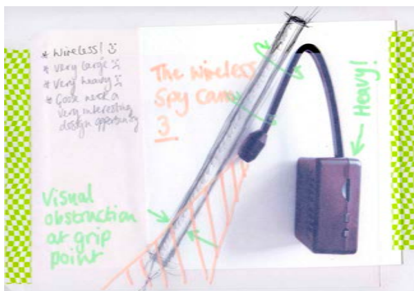
Figure 15 Excerpt from the author's sketchbook, detailing experiments with miniature spy camera type 3.
