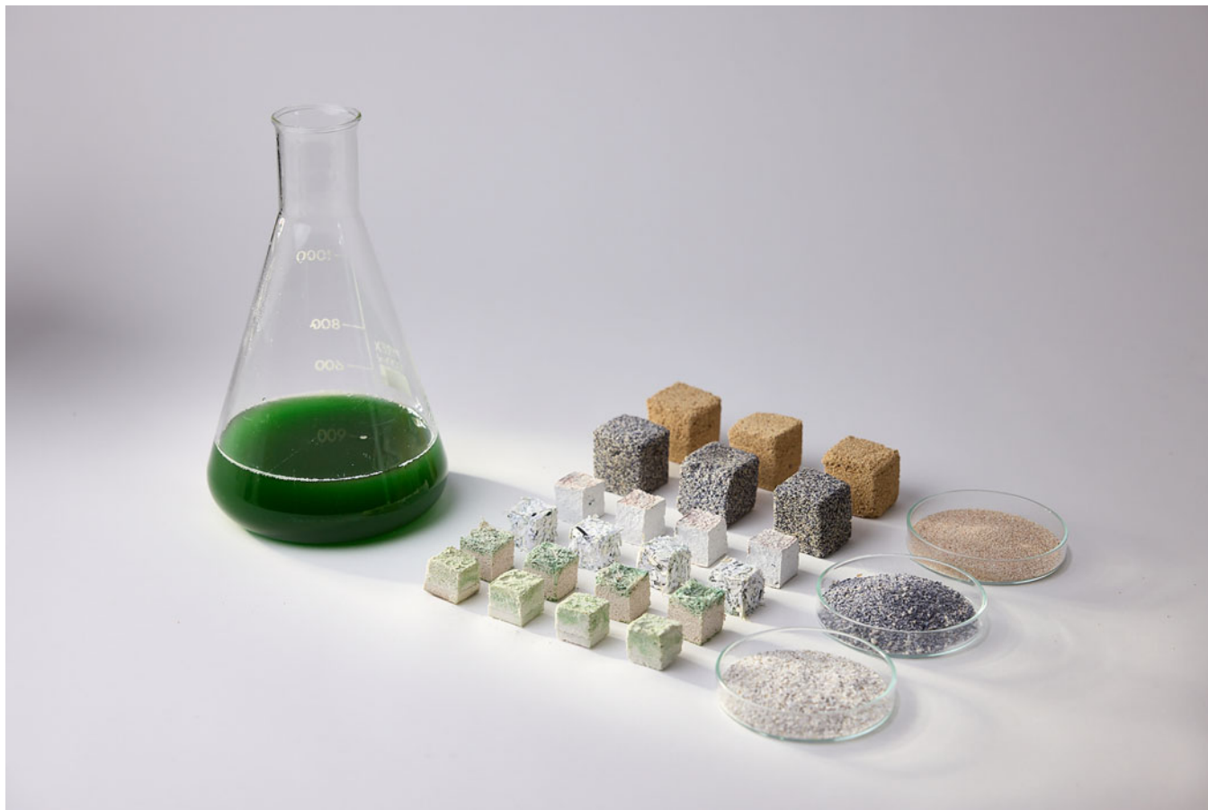
Figure 8. Representative photosynthetic biomineralisation material sample collection, showing cyanobacterial culture, processed waste-derived materials and fabricated samples developed through the three biofabrication workflows, reproduced from Shin et al. (2026). Photograph by Paul Cochrane.
