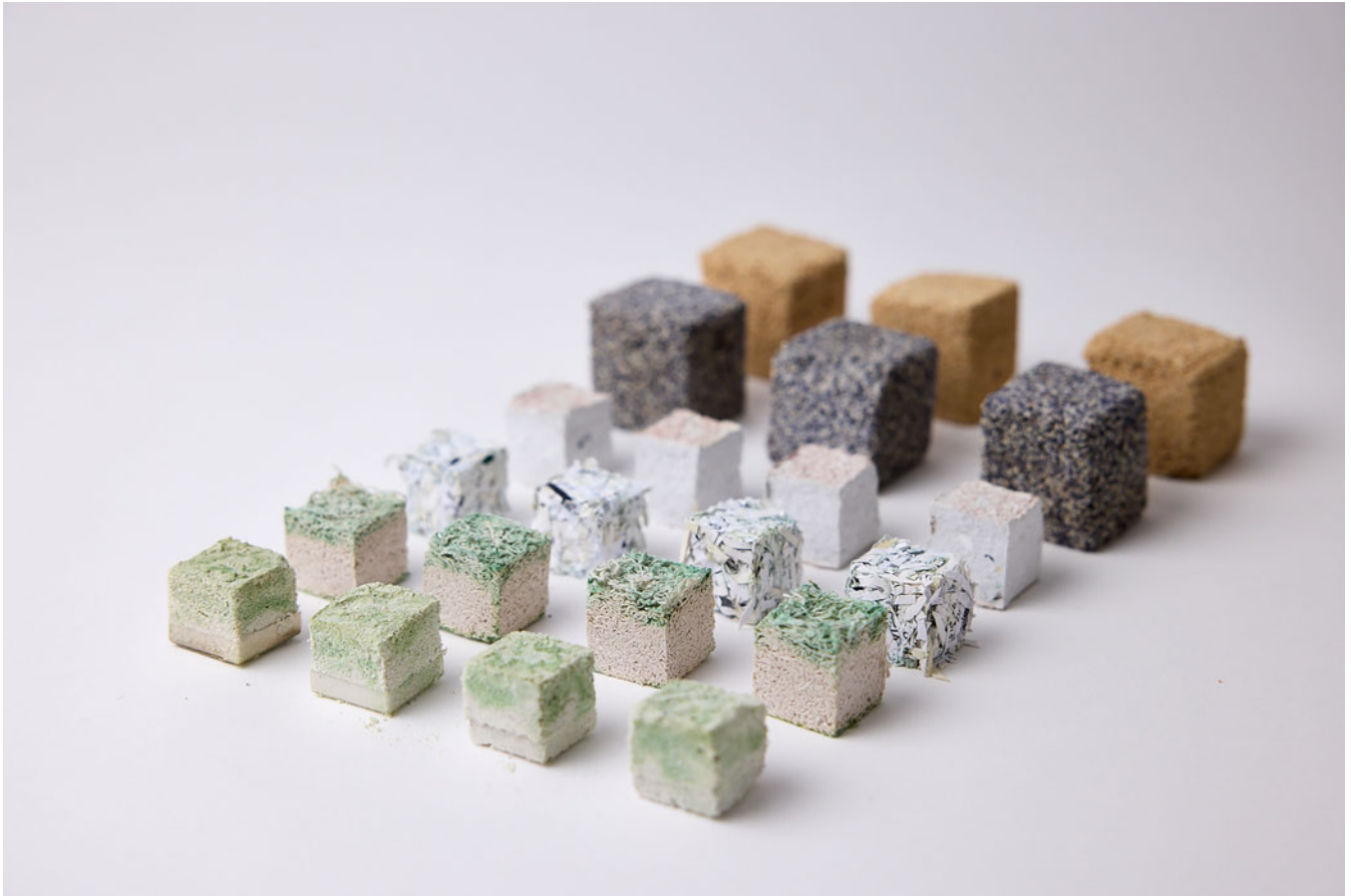
Figure 10. Selected dried material samples from the three workflows, showing visible variation in material appearance and structural cohesion across waste-derived material types. Photograph by Paul Cochrane.
