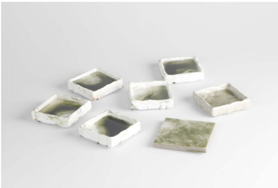
Figure 12. Colour variations of algae pigment coating on tiles.
