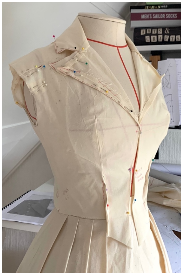
Figure 4.22: Riding habit jacket toile with adjustments marked using pins and pen.
