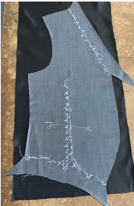
View of the front placed on lining for cutting out the lining
