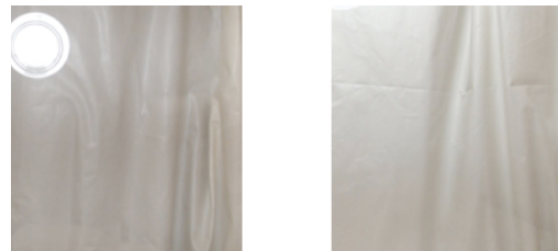
Figure 4 (left): A single light source centrally located below the textile, mounted next to the camera. This caused unrealistic reflection of the lamp but was successful at highlighting gloss. (right): Lighting from both above at 180 degrees and centrally below with lamp moved outside the filmed area. Less successful at highlighting gloss surfaces
