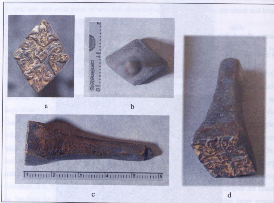
Figure 21 - Tool 10: a) photograph of face, b) view of the rear side, c) side view, d) general view
