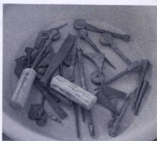
Fig.4 The tools discovered at Saint Catherine's were put in a bucket and handed to me for examination. They include rolls, corner-pieces, centre-pieces, small hand tools, fillets and creasers.
