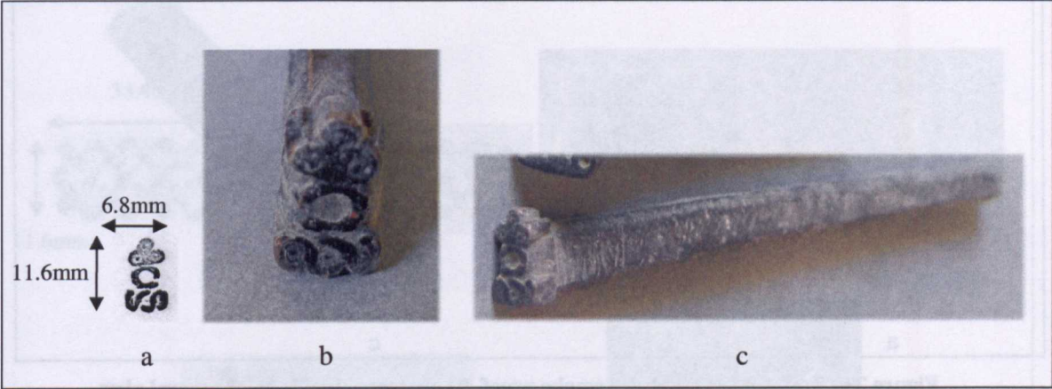
Figure 27 - Tool 14: a) actual size smoke proof, b) photograph of face. c) general view
