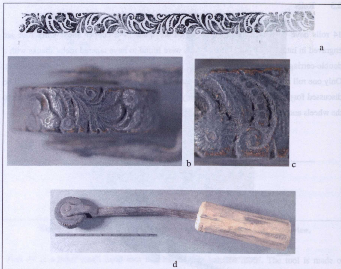
Figure 32 - Tool 18: a) actual size smoke proof, b) photograph of wheel, c) detail showing casting holes, d) general view
